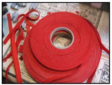
The original thickness of felt is used as a starting point in choosing a felt which will provide a snug fit for the keys without being so tight as to cause binding.
