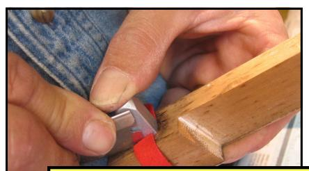
After the felt is inserted into the key, a sizing caul (a precision fitting device) is used to hold the felt in place while a razor is used to slice it precisely to the correct length.
